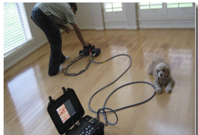
Figure 3. Picture showing the 1500 MHz GPR survey in the living room. The GPR data was collected at every 6 inch.
